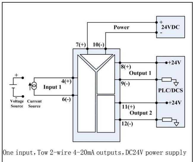
Note: The connection diagrams given in this manual are typical. When installing, please refer to the connection diagram on the product.
